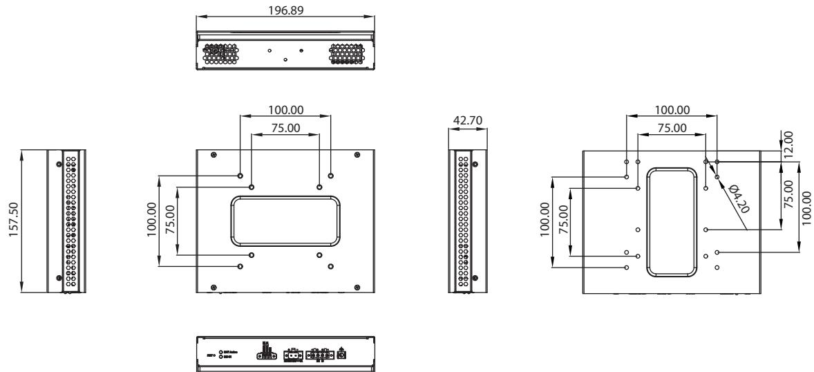
Max.depth for VESA Mounting screws is M4\*8(mm)
