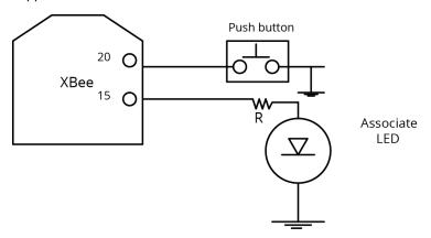
To support the Commissioning Pushbutton and its associated LED functions, connect a pushbutton and an LED to device pins 20 and 15 respectively.
