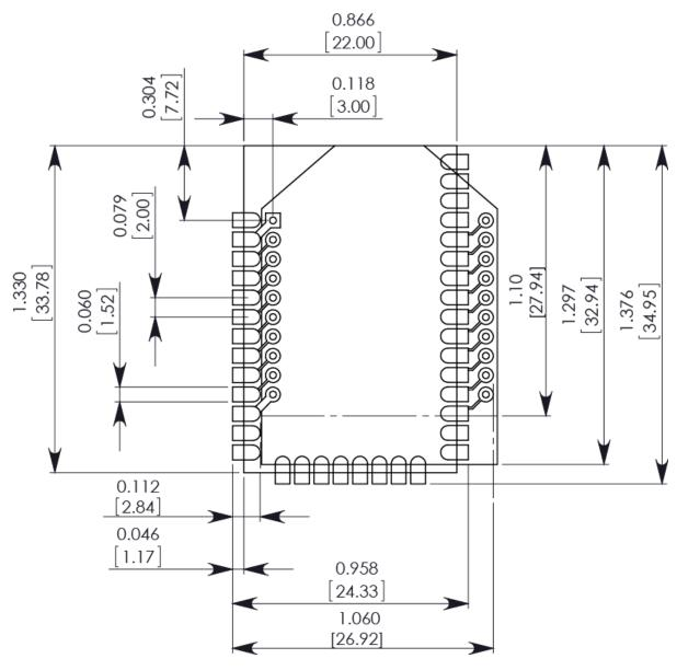
The round holes in the diagram are for the TH design, and the semi-oval pads are for the SMT design. Pin 1 of the TH design is lined up with pad 1 of the SMT design, but the pins are actually offset by one pad; see Pin mapping. By using diagonal traces to connect the appropriate pins, the layout will work for both devices.
