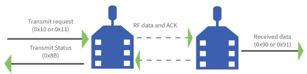
The device sends the 0x8B Transmit Status frame at the end of a data transmission unless you set the frame ID to 0 in the transmit request. If the packet cannot be delivered to the destination, the 0x8B Transmit Status frame indicates the cause of failure.
