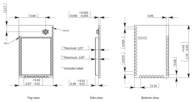
The drawings below show the XBee through-hole model
